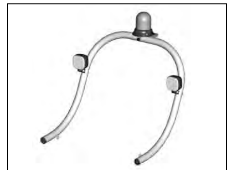
Rollbar lowered of 120 mm
