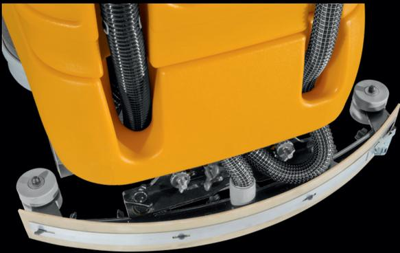
The new and innovative “low-chamber” squeegee is the result of comprehensive studies on the flow dynamics of the dirty matter collected. This new type of squeegee, shaped like an arc, generates a higher negative pressure inside the collection chamber. This helps to improve drying performance while the machine moves and reduces
