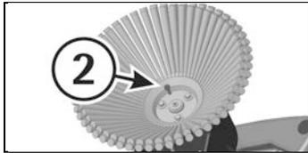
To assemble the brush, properly tighten the screw (2)
