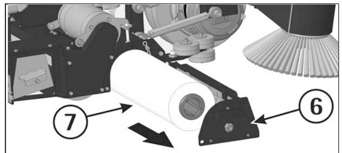
11. When reassembling the brush, insert it where the position is deeper (about 1.5" - 40mm). The side has to be towards the support plate.
