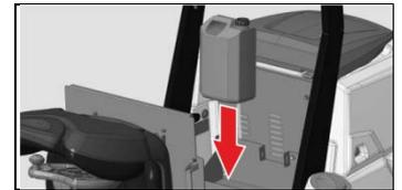
Remove the cap of the tank and replace it with the adapter. The hose has to touch the tank bottom.
