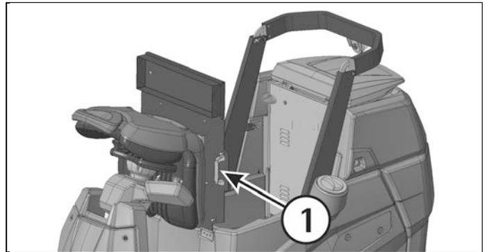
If the machine is equipped with the optional 3SD water system, it is necessary to take off the support of the detergent tanks after lifting the seat base. To remove the support, unscrew the 6 fixing screws.
