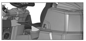
Screw the solution tank cap.
