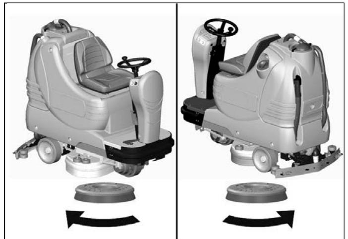
For a longer life of the brushes we suggest to invert daily their position. Whenever brushes result to be deformed we suggest to reassemble them in the same position, in order to avoid that the different inclination of the bristles causes excessive motor overload or troublesome vibrations.
