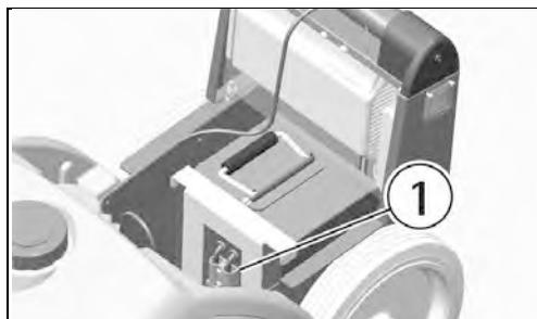
**DISASSEMBLY OF THE BATTERIES (STANDARD AGM VERSION)**
