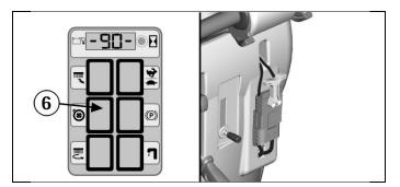
Check that the red connector of the suction motor (1) is correctly plugged in.
