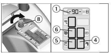
Models equipped with the 3S system (optional), it is necessary to press the suitable switch to activate the detergent solution supply by choosing between the traditional adjustment system through the solution valve or the system of fixed optimum supply (see under "3S SYSTEM SOLUTION SAVING SYSTEM").
