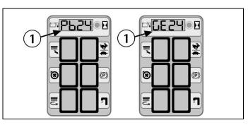
The batteries charge level indicator (1) is digital and indicates the percentage of the battery charge. 90 is the maximum charge, down to a minimum of 10, indicating every 10% decrease. When the charge level reaches 20%, the display starts blinking indicating the end of the battery charge.
