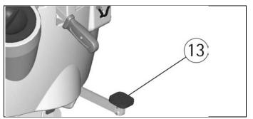
With the brushes base group in lifted position, insert the brushes into their plate seat underneath the brushes base turning them until the three metal buttons are properly seated in their slots; rotate energically the brushes to push the button towards the coupling spring until they get blocked.
