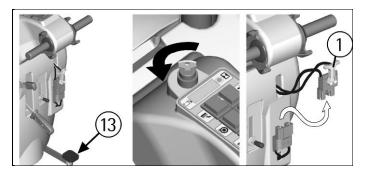
With the brushes base in lifted position, turn the brush in its 4. rotating sense as indicated in the figure, until it is released from the brush holder plate seat as indicated in the figure. The figures show rotating sense for brushes release.
