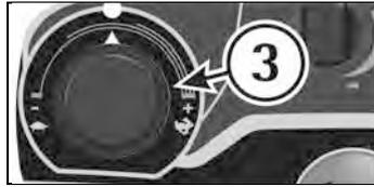
If backward movement is selected the brush base will stay down, the squeegee will lift up and the suction motor will shut itself. When the forward movement will be selected again the squeegee will go down and the suction motor will turn back on.
