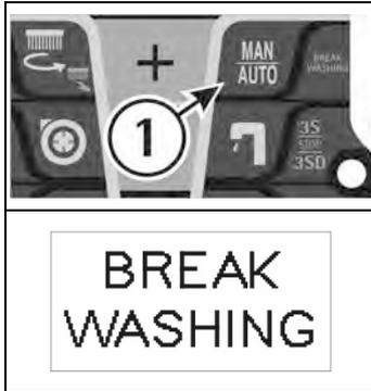
This way automatically the brushes lift, the solenoid valve shuts down and it is possible to finish the drying operation for a total time of about 15 seconds, afterwards also the squeegee is lifted and the suction stops.
