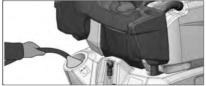
On the rear part of the machine is placed a level hose that permits to see easily the solution quantity inside the tank both during the filling of the solution and during the working.
