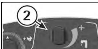
3. Open the valve (2) for the solution draining.
