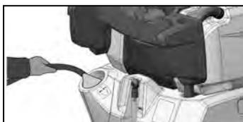
4. Clean the tank with a water jet.
