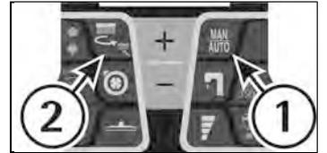
On the display value P1, P2 or P3 will blink. Press the buttons (+) and (-) to select the pressure, the value will set once it will stop blinking on the display.
