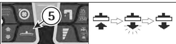
6. While running the first meters check that the squeegee adjustment guarantees a perfect drying action and that the detergent solution flow is appropriate. It has to be sufficient to wet the floor uniformly avoiding the leakage of detergent from
