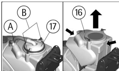
5. Empty the recovery tank into appropriate containers, according to the standard norms for the liquid disposal.
