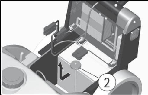
5. Take off the other battery (4) making it slide forwards in the battery compartment, then take it off.
