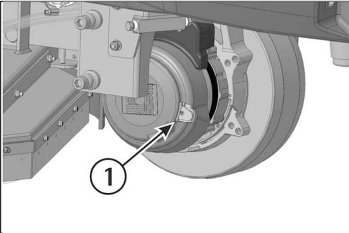
3. Release the machine from the wooden brackets by moving it backwards, as indicated in the figure, avoiding heavy contacts to mechanical parts.
