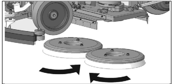
For a longer life of the brushes we suggest to invert daily their position. Whenever brushes result to be deformed we suggest reassembling them in the same position, in order to avoid that the different inclination of the bristles causes excessive motor overload or troublesome vibrations.
