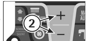
After a few seconds the value stops blinking and the detergent percentage is selected. With the value 0% only water is used for washing.
