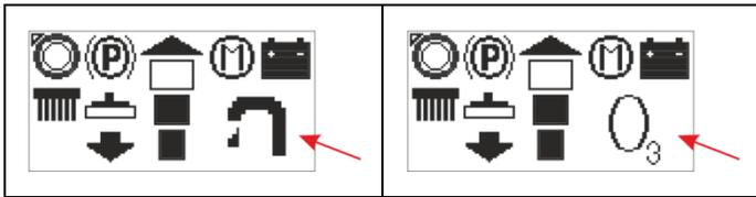
When the O3 icon stops blinking the system is being selected.
