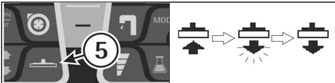
6. While running the first meters, check that the squeegee adjustment guarantees a perfect drying action and that the detergent solution flow is appropriate. It has to be sufficient to wet the floor uniformly avoiding the leakage of detergent from the splash guards. Always consider that the correct quantity of solution detergent depends on the type of floor, dirtiness and machine speed.
