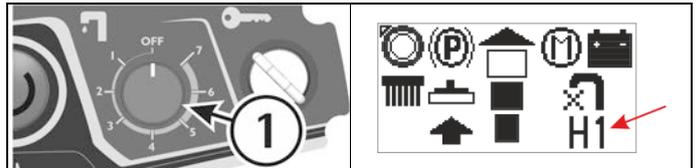
When in standard mode the detergent solution flow stays the one that has been set.
