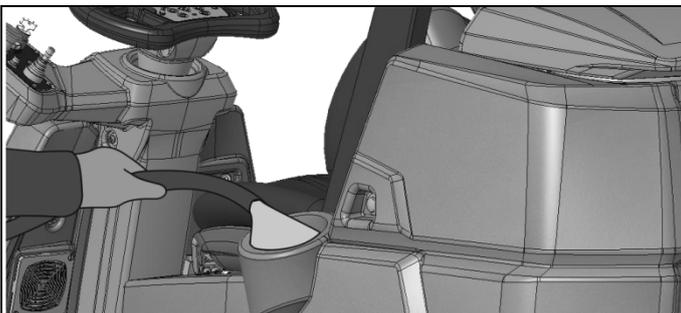
Screw the solution tank cap.
