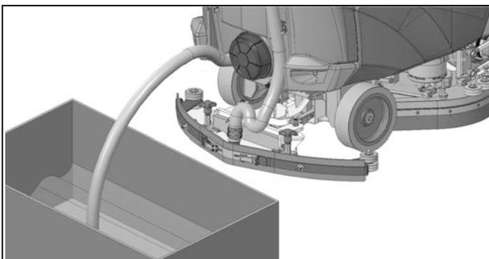
3. After the tank is completely drained, take off the drain box (1) by releasing the lever (2) and unscrew the cap (3).
