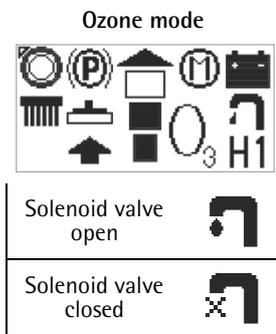
If the machine is equipped with the Ozone system and an optional hydraulic circuit (3S or 3SD) and is chosen to combine the Ozone with one of these two systems, the display will show the following inputs:
