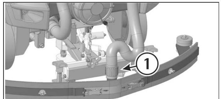
2. Wash the inside of the hose with a water jet.
