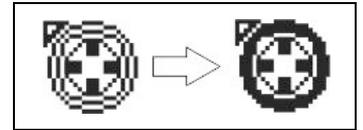
8. Check that the suction motor cap is closed properly.
